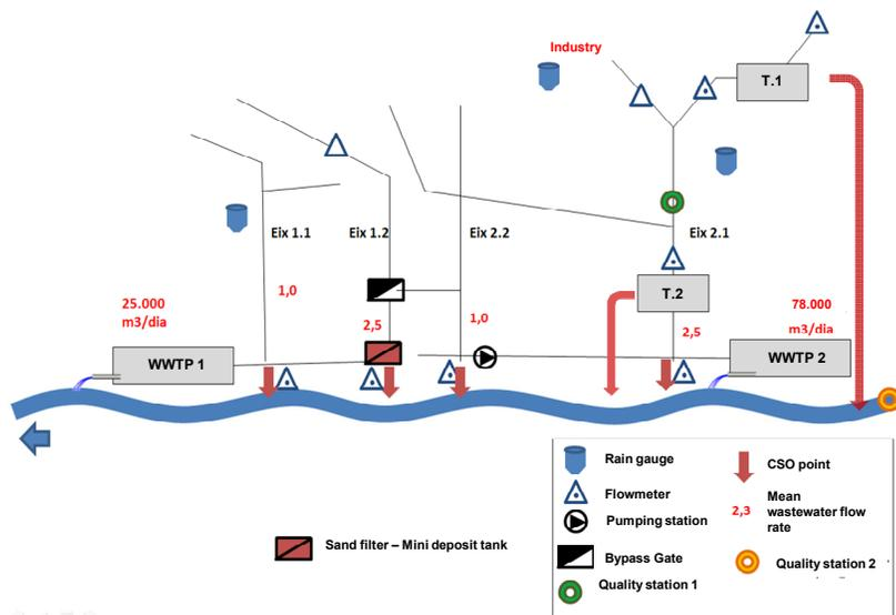
**Figure 3.** Virtual system scheme.
