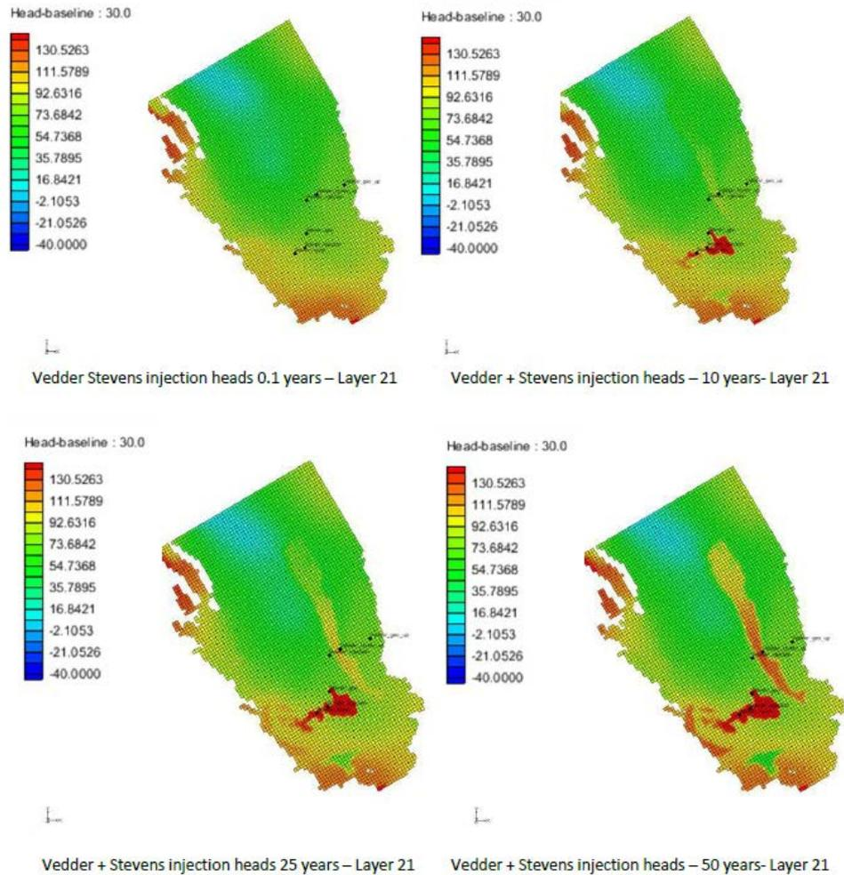
Figure 3. Vedder and Stevens injection head contours (meters) for Layer 21 at 0.1 years, 10 years, 25 years, and 50 years. Plots show distinct head increases which are more pronounced in the shallow Stevens formation injection.
