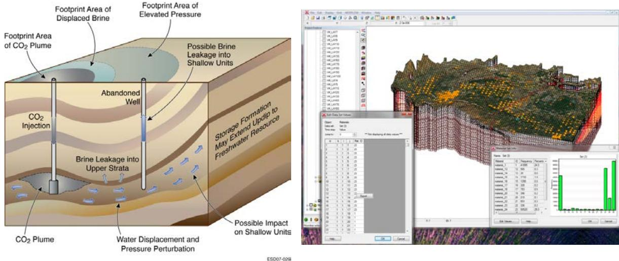
Figure 1. (a) Schematic showing different regions of influence related to CO<sub>2</sub> storage (Birkholzer et al., 2008, 2009; Zhou et al, 2011). (b) CVHM-Kern-FMP3 model domain and extended vertical mesh using Aquaveo GMS software (Quinn et al., 2013).
