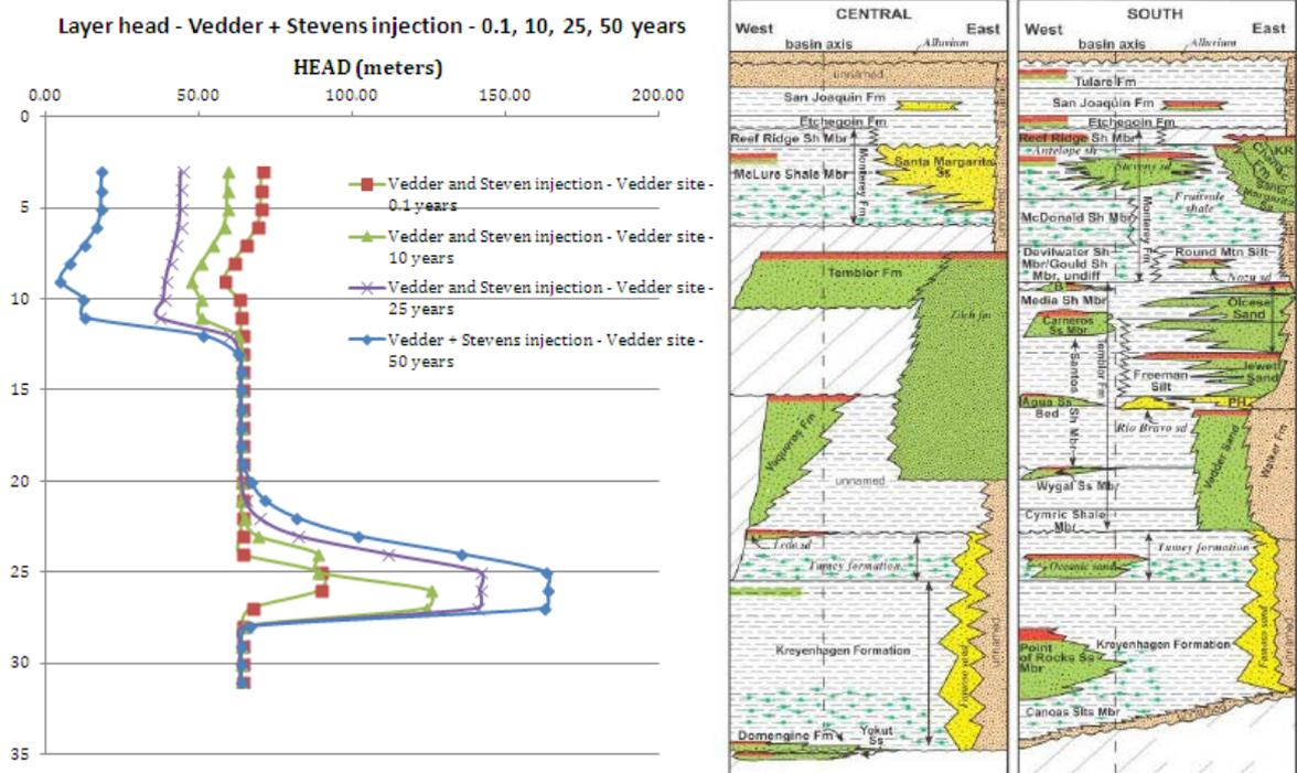
Figure 2. (a) Head profiles for the injection simulation into the Vedder and Stevens sand formations observed at the Vedder site for 0.1, 10, 25 and 50 years. Depth in the vertical axis is represented as “layer number.” There are 31 vertical layers. (b) Generalized stratigraphic section for the CVHM-Kern model region showing location of Vedder and Stevens sand formations (Quinn et al., 2013).
