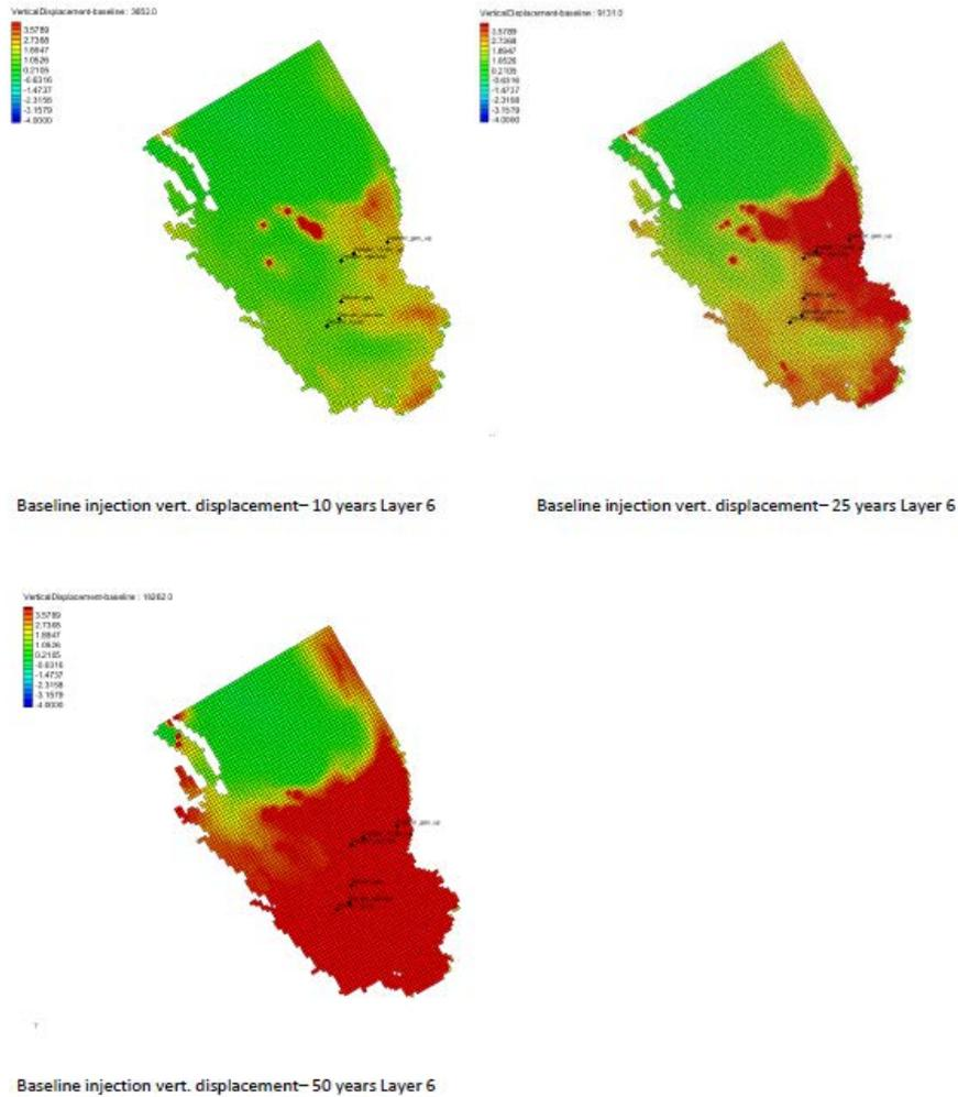
Figure 5. Baseline vertical displacement contours (meters) for Layer 6 at 10 years, 25 years, and 50 years. Positive values indicate subsidence, negative values indicate uplift.
