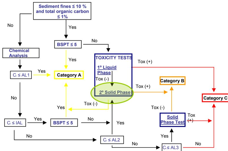
**Figure 1.** Spanish dredged material management framework represented as decision making flowchart proposed in 2008.  $C_i$  – concentration of the  $i$ -th contaminant; BSPT – response in Microtox® basic solid-phase test; AL1-AL3 and IAL – four different sediment guidelines adopted in Spain; categories A-C characterize sediment contamination state and also represent management options relative to dredged sediment.
