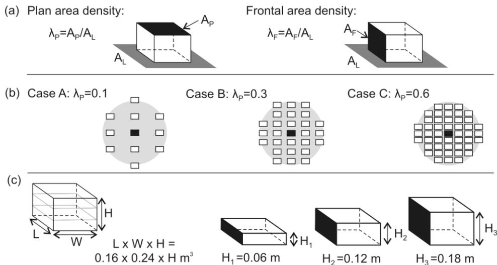
**Figure 1.** (a) Definition of plan area density and frontal area density; (b) variation of plan area density ( $\lambda_p$ ) from 0.1 (case A) to 0.6 (case C); (c) variation of building height from 0.06 m ( $H_1$ ) to 0.18 m ( $H_3$ ).
