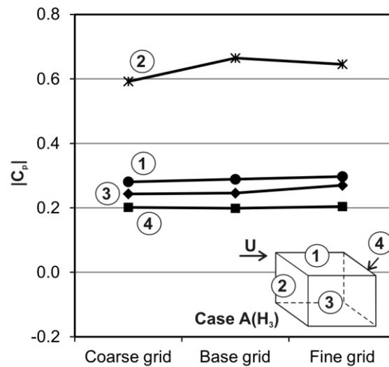
**Figure 4.** Grid sensitivity analysis for case A(H<sub>3</sub>): comparison between the absolute values of the mean wind pressure coefficients on the walls of the central building obtained with three grids.
