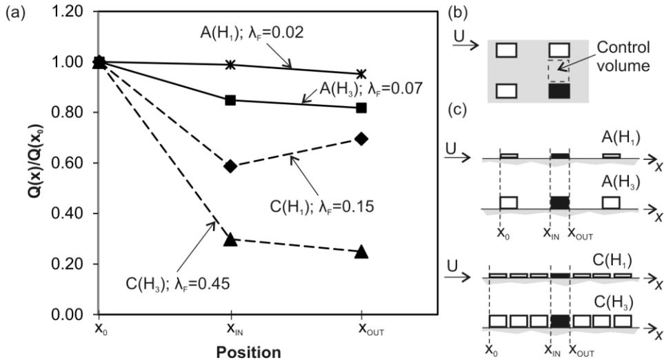
**Figure 6.** (a) Comparison of the ratio  $Q(x)/Q(x_0)$  between the ventilation rates at the first and the central building positions; (b) Definition of a control volume of interest, ground plane; (c) Sections used for calculating the ventilation rate in the different urban configurations, vertical section.
