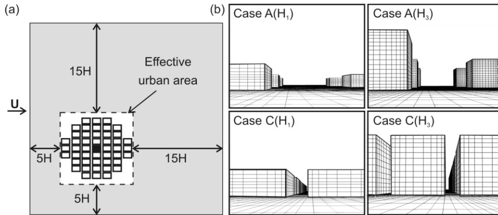
**Figure 3.** (a) Computational domain size for the cases C(H<sub>1</sub>) and C(H<sub>3</sub>); (b) Perspective view of the computational grids used for the simulations.
