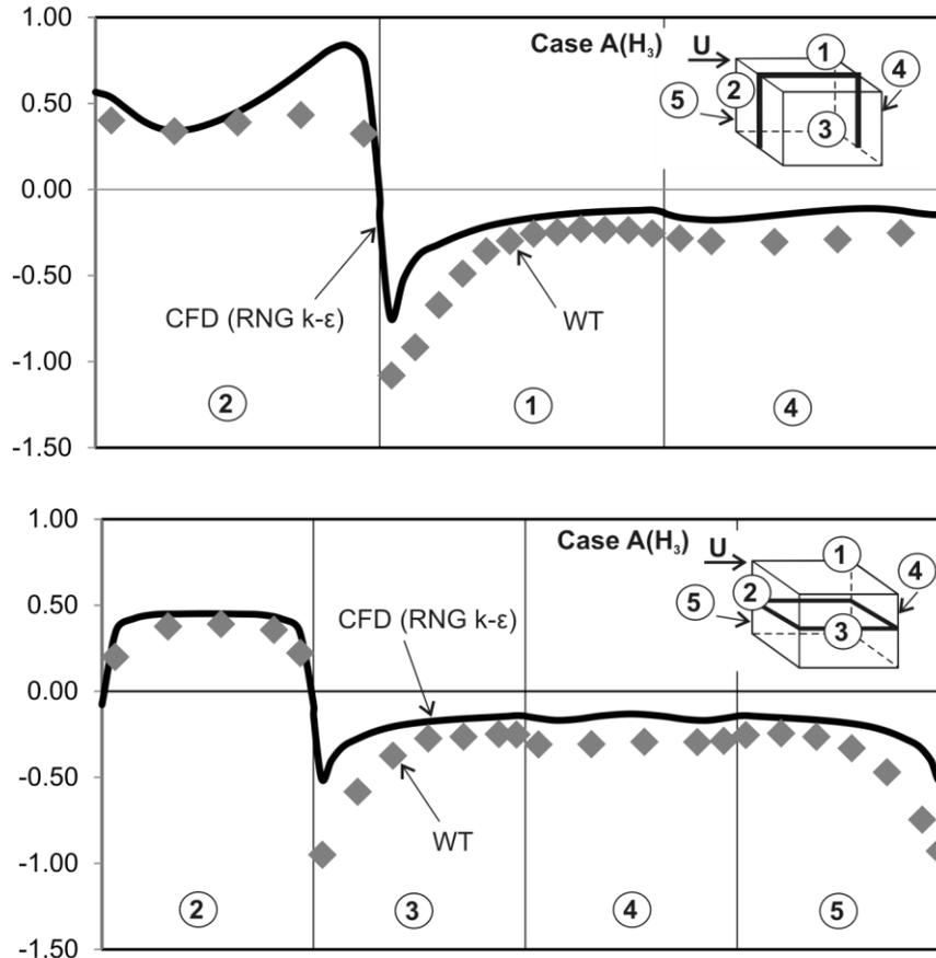
**Figure 5.** Comparison of numerical and experimental results for case A(H<sub>3</sub>) in terms of mean pressure coefficients along the midlines of the central building.
