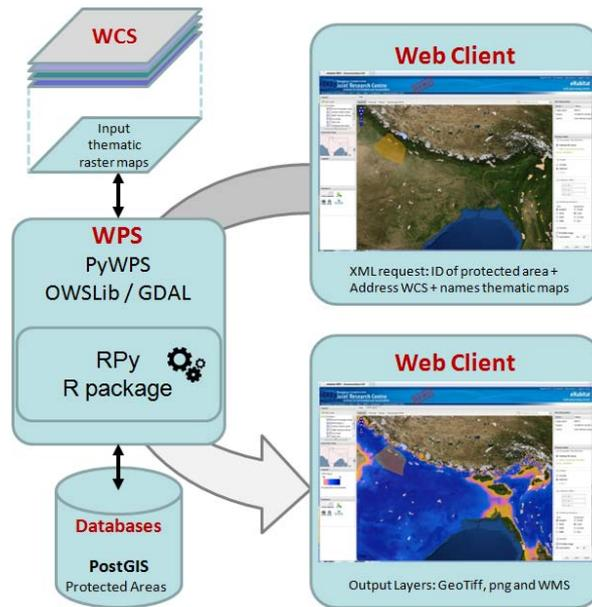
**Figure 2.** Schematic representation of the architecture of the eHabitat WPS.
