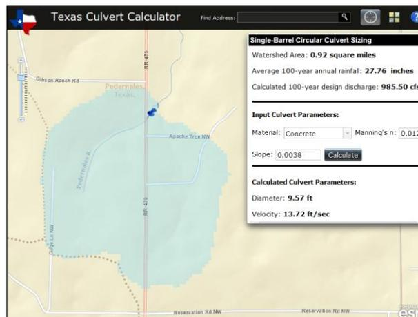
Figure 4. Interactive runoff calculation and culvert sizing application
