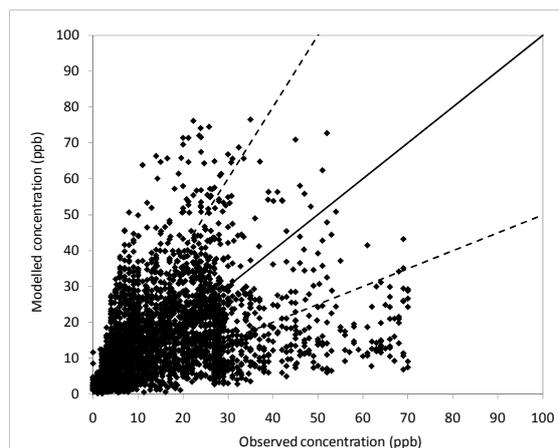
**Figure 2.** Scatter plot of observed and modelled hourly NO<sub>2</sub> concentrations (N=2909). The lines 2:1, 1:1 and 1:2 are included
