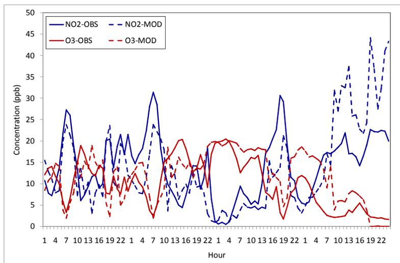
**Figure 5.** Time series of observed and modelled NO<sub>2</sub> and O<sub>3</sub> concentrations (ppb) during four days (4-7 September 2001) at the UB site.
