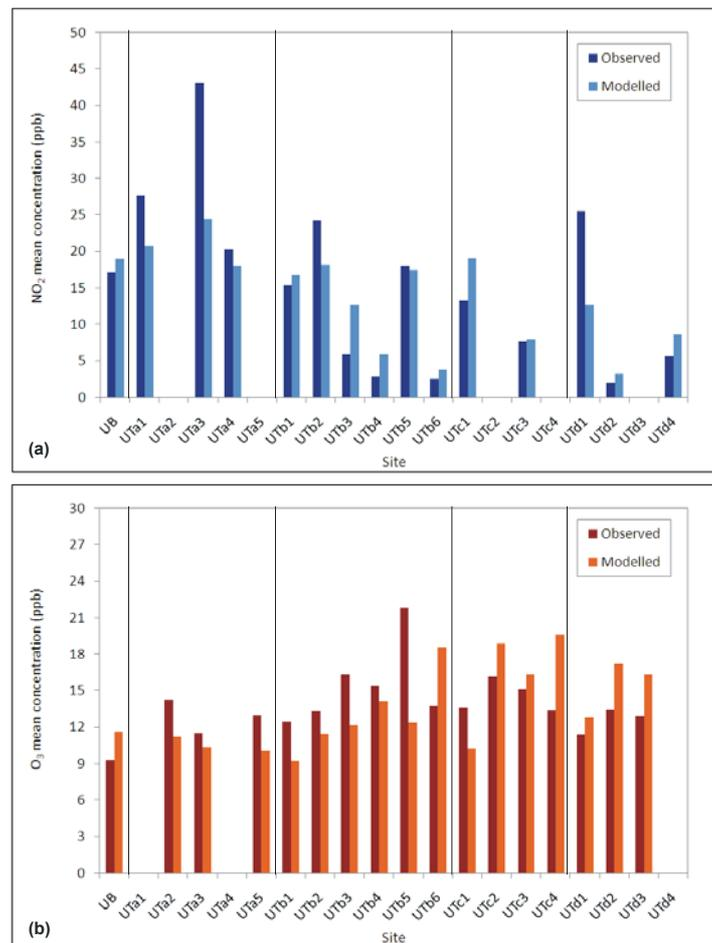
**Figure 4.** Comparison between observed and modelled mean concentrations: (a) NO<sub>2</sub> and (b) O<sub>3</sub>.
