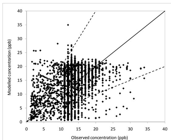
**Figure 3.** Scatter plot of observed and modelled hourly O<sub>3</sub> concentrations (N=3100). The lines 2:1, 1:1 and 1:2 are included
