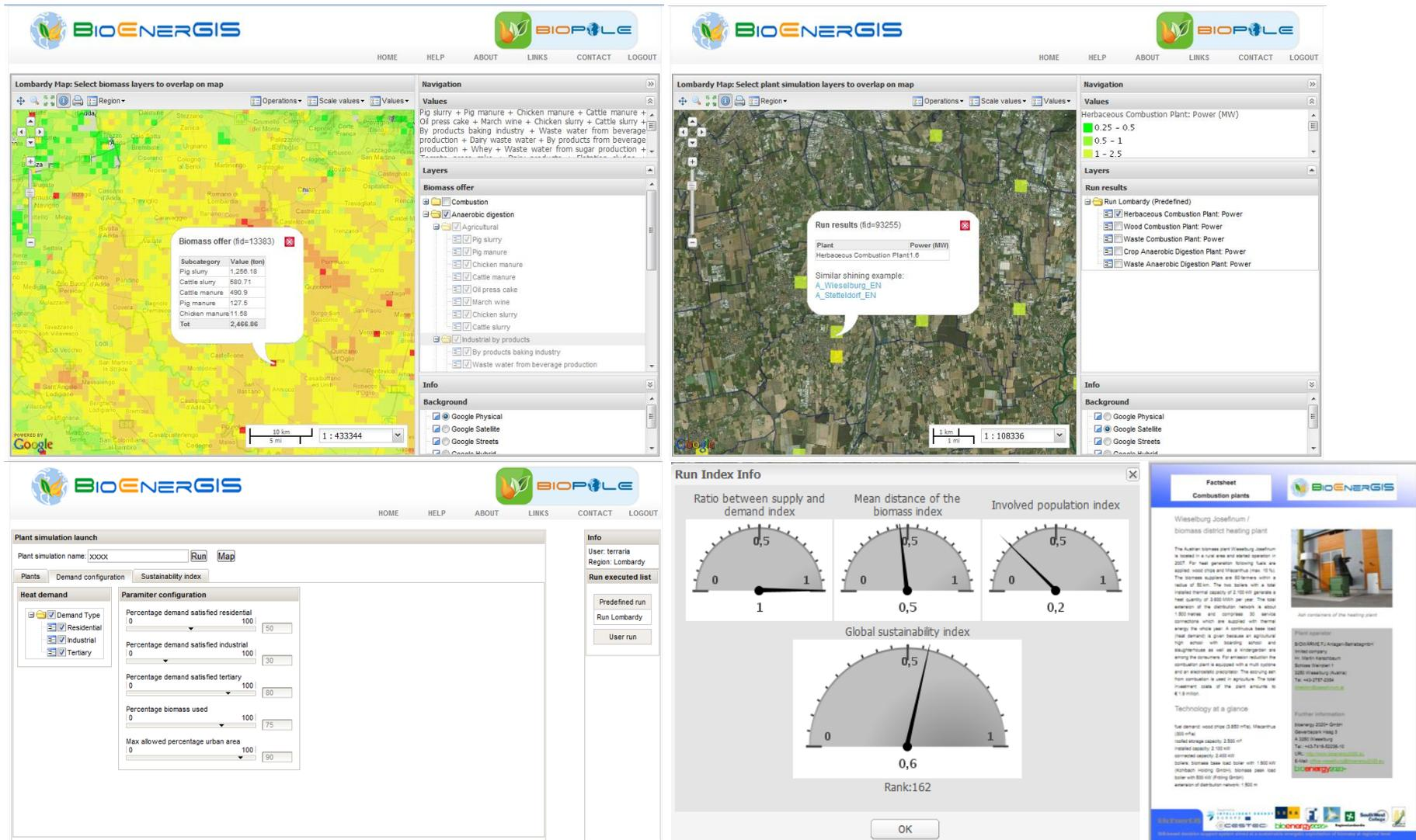
Figure 3. BIOPOLE screenshots examples: offer (biomass availability) analysis (top left), simulation plant results (top right), simulation parameters (bottom left), sustainability dashboard (bottom middle) and plant factsheet (bottom right).
