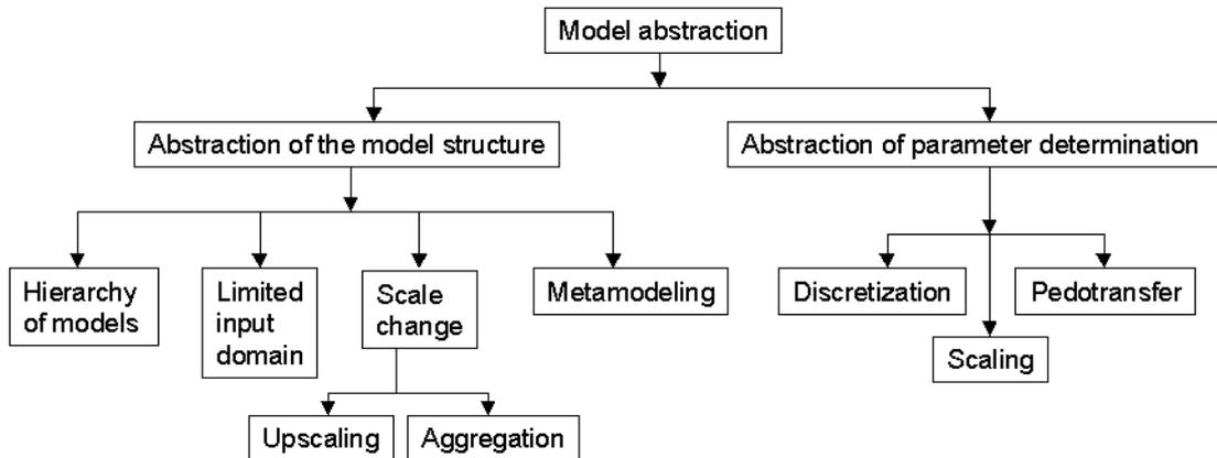
**Figure 1.** Categories of model abstraction techniques relevant to flow and transport modeling in subsurface hydrology
