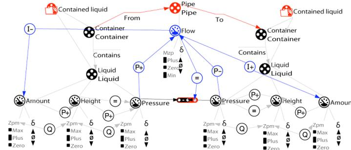
Figure 1: Liquid flow includes 2 Contained Liquid IMFs, a Pipe, and the configurations as conditions, and flow, its calculation and causal relations as consequences.
